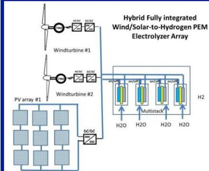
**Objective:** Experimental facility for hydrogen generation (multi stack) directly coupled to hybrid renewable generation (solar PV and/or wind) and using a single modular electronic power conditioning system.
