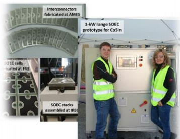
Image of the first prototype of SOEC fabricated in collaboration with the Catalan companies FAE and AMES
